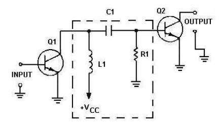
Figure 1-11.—Impedance-coupled transistor amplifier.
