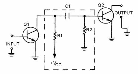
Figure 1-10.—RC-coupled transistor amplifier.
