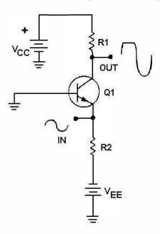
Figure 1-5.—A simple class AB transistor amplifier.
