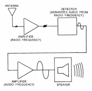
Figure 1-2.—Amplifiers as used in radio receiver.
