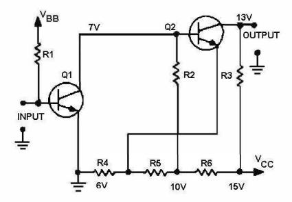
Figure 1-9.—Direct-coupled transistor amplifiers.
