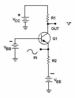
Figure 1-7.—A simple class C transistor amplifier.
