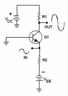
Figure 1-4.—A simple class A transistor amplifier.
