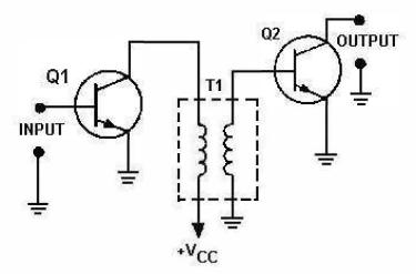
Figure 1-12.—Transformer-coupled transistor amplifier.
