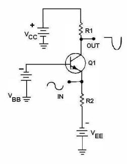
Figure 1-6.—A simple class B transistor amplifier.
