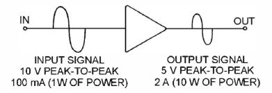
Figure 1-3B.—Block diagram of voltage and power amplifiers.
